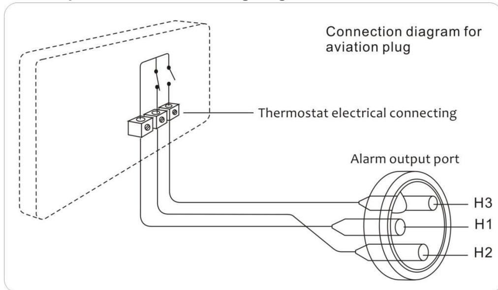
Note: The alarm output port is connected with a set of normally open and normally closed contacts of the relay inside the machine. The working current should be smaller than 3A while the working voltage should be smaller than 300V.
